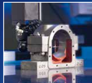
Defined random sampling using 2D and 3D measurements and careful final inspection guarantee HFB's exceptional product quality
